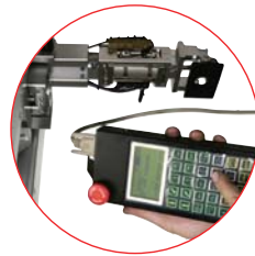
Remote vertical and horizontal adjustment, standard on BE-1100 and -1300
