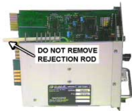
Figure 3 - Rejection Rod on High Power Modules (Do Not Remove)
