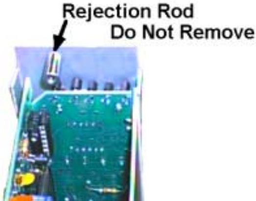
Figure 2 - Rejection Rod on Low Voltage Modules (Do Not Remove)
