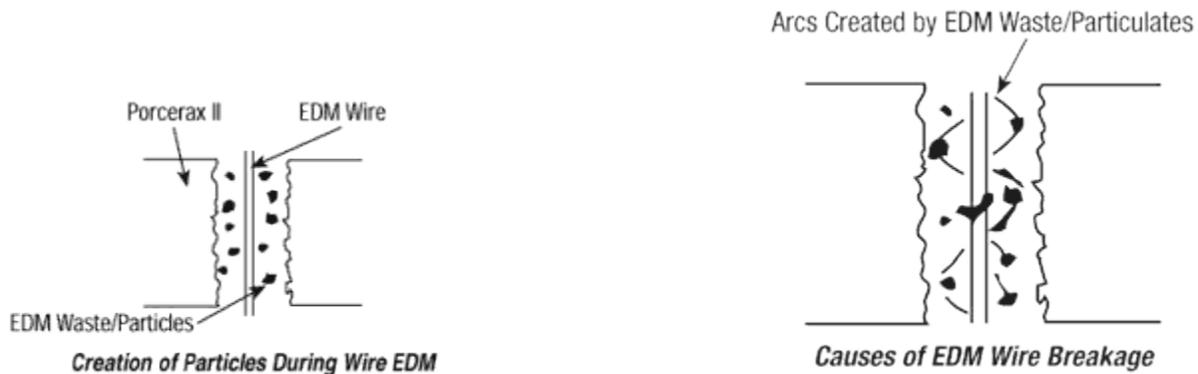
The illustrations above show how particles created by the wire EDM process carry the electrical current across to the work-piece, creating the potential for a discharge that can break the wire. Increasing the wire winding speed not only greatly reduces the potential for wire breakage but also increases machining times.
