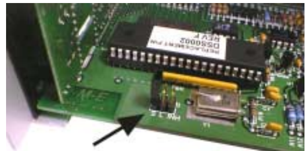
Figure 9 - 100% Power Jumper (J1) Location
