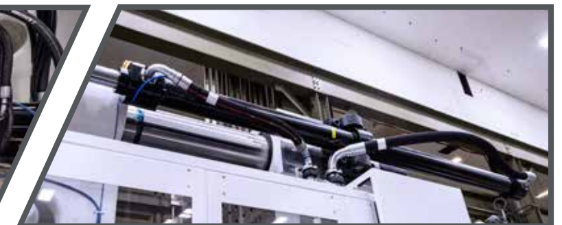
Traverse Cylinders with Trunnion mount
